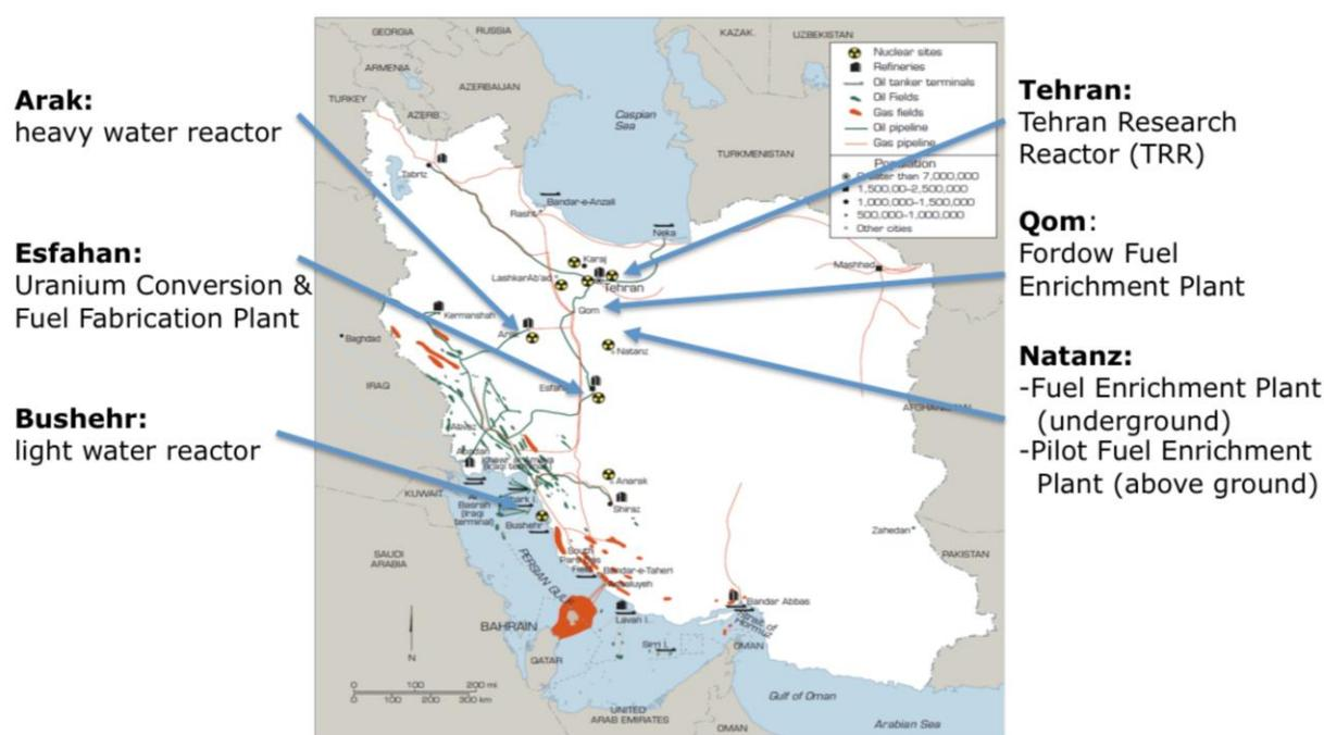
*Fuel Enrichment Plant—Natanz.* The Fuel Enrichment Plant (FEP) is a below-ground enrichment facility located at Natanz. Since 2002, it has been the hub of Iran’s enrichment program. It consists of two underground halls designed to hold a total of 50,000 centrifuges.
